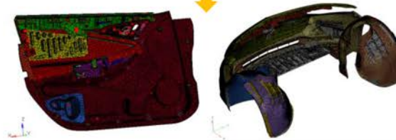
Complete assembly with connections and contacts for interiors and exterior plastic parts
