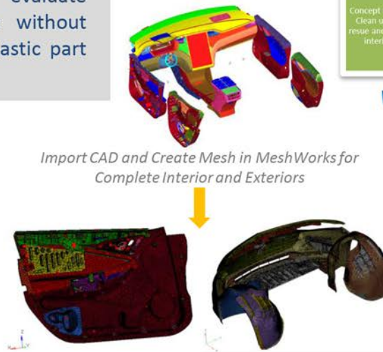
Complete assembly with connections and contacts for interiors and exterior plastic parts
