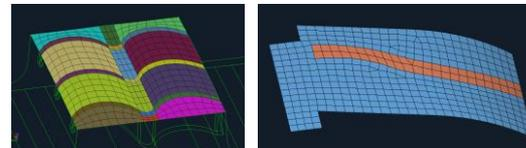
Surface mesh to capture the Tire tread features
